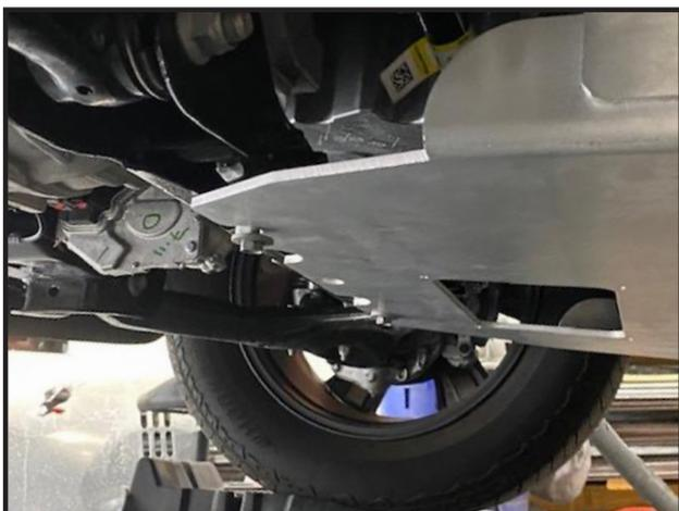
3. The front felt bracket may be removed or left in place. If keeping the engine felt liners you will need to leave it in place. Loosen the M10x1.5 Bolts so there is approximately a 1/2" gap. You will slide the front slots of the transmission skid plate onto these bolts. If the factory felt liner bracket is left in place, we recommend removing the spring clips to prevent a rattle. We are now including M10 button head bolts which can be installed instead of the M10 hex bolts if desired.
