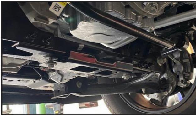
2. Remove the Factory Felt Covers if not already removed including the side brackets from the frame.
